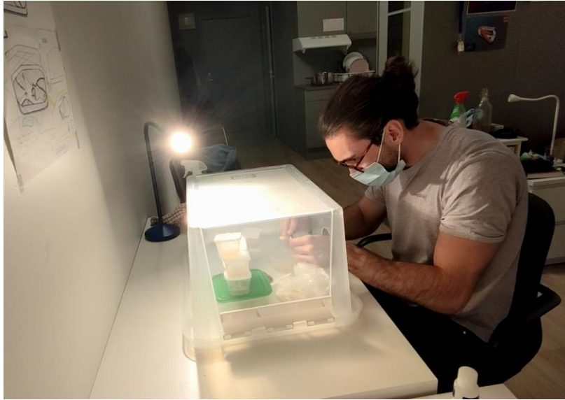
Fig. 55. Inoculation of the moulds with T.versicolour and hemp.
