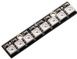
Figure 28. NEO Pixel Stick Light with 80 5050 RGB lights (Adafruit).
