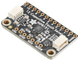
Figure 30. Adafruit MPR121 12-Key Capacitive Touch Sensor (Adafruit).
